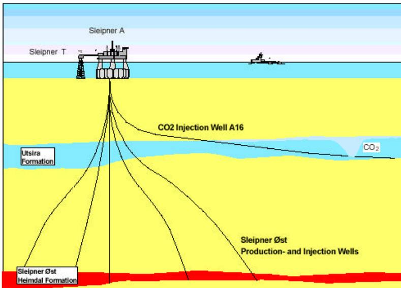
**Figure 2: CO<sub>2</sub> reinjection from the Sleipner platform (Kaarstadt, IPCC).**
